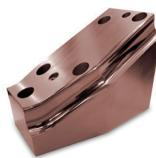
**Red Speed Lafer** is a **TiAlCN coating** used successfully in wet chip removal on medium low strength steels, both in interrupted and continuous cutting conditions. Its **multilayer structure** has been developed to ensure maximum adhesion and to withstand the most severe mechanical stresses, while the red functional outer layer **guarantees a lower resistance to chip sliding**.
