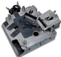
**Kronos** coating, based on **AlCrN**, is the Lafer solution for die-casting Aluminium, Zamak and Magnesium. its composition is ideal for solving **metallization problems**. It allows you to combine the **high wear resistance**, typical of coatings containing Chromo, with that at high temperatures, typical of coatings containing aluminium.
